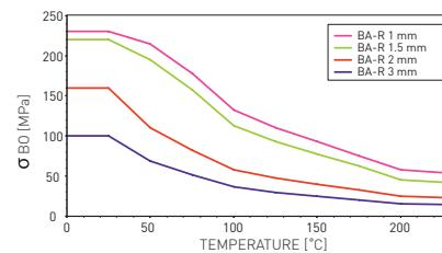
σ<sub>BO</sub> diagrams represent σ<sub>BO</sub> values for different gasket material thicknesses. These values indicate the maximum in-service compressive pressures which can be applied on the compressed gasket area in-service without destroying the gasket material.
